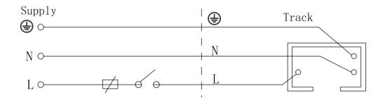
1-phase, 1-circuit, 230V AC, 10A, 3kVA
